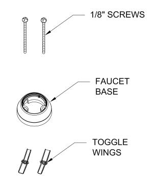
3. Assemble the 1/8" Screws & Toggle Wings into the Faucet Base. Adjust the Wings approximately 1" plus the thickness of the mounting surface away from the bottom of the Faucet Base.
